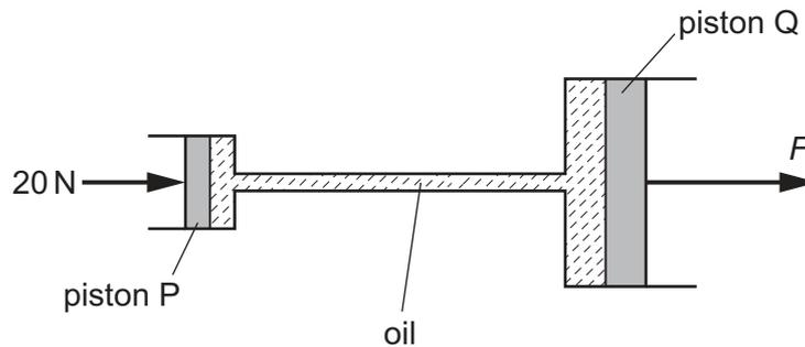
Piston P has an area of  $5.0 \text{ cm}^2$  and piston Q has an area of  $25 \text{ cm}^2$ .
